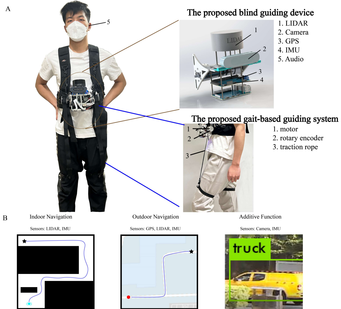
Figure 1: Overview of the Proposed Blind Guiding Device. (A) The device incorporates multiple sensors and our innovative gait-based guiding system. (B) Various sensors are employed to capture environmental information across different scenarios.
