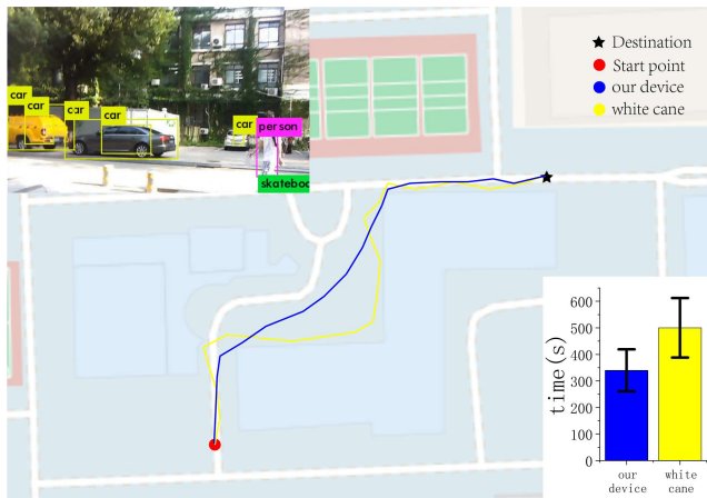
Figure 8: Outdoor Navigation Experiment. The top left corner features a demonstration of our computer vision. The bar chart with error bars in the bottom right corner illustrates the time spent by our device and a white cane.
